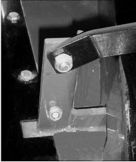
**Step 2**: Connect all braces at the top of the A-frame with an M12 bolt, spacer, hitch connection, and locking nut. See below picture:
